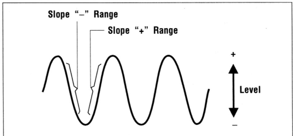
**Fig. 14. Function of slope and level controls.**
